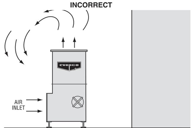
Figure 34 - Wind Effect with Top of Unit Lower than Top of Wall
