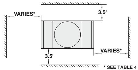
Figure 57 - Minimum Clearance Dimensions Induced Draft Crossflow Units
