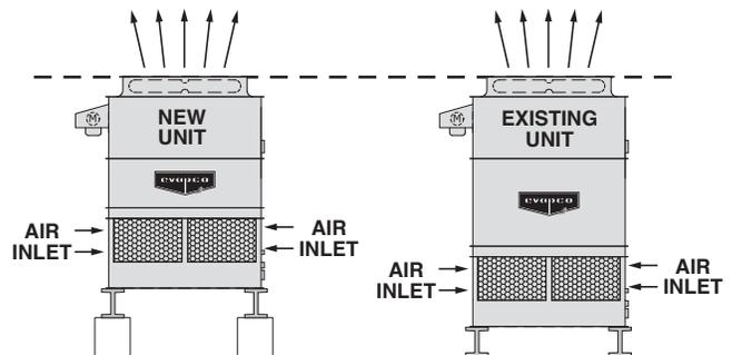
Figure 22 - Expansion to an Existing Installation
