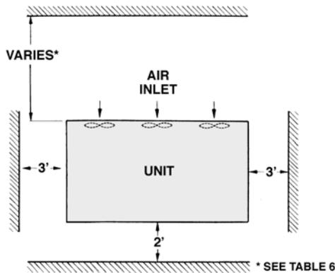
Figure 54 - Minimum Clearance Dimensions Forced Draft Units
