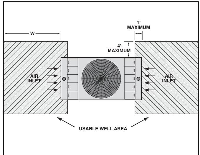
Figure 30 - Well Installation
