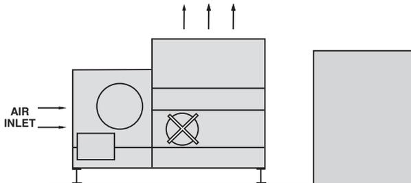
**Figure 37** - Installation Next to Wall, Best Orientation
