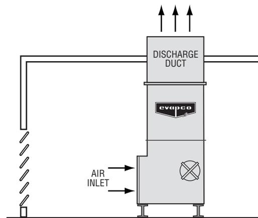
**Figure 50 - Indoor Installation with Floor Acting as Plenum**
