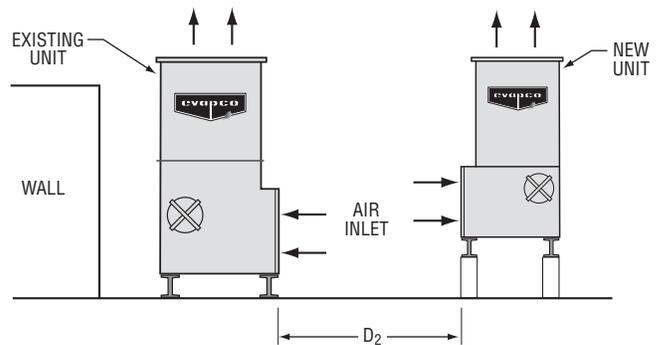
**Figure 53 - Expansion to an Existing Installation**
