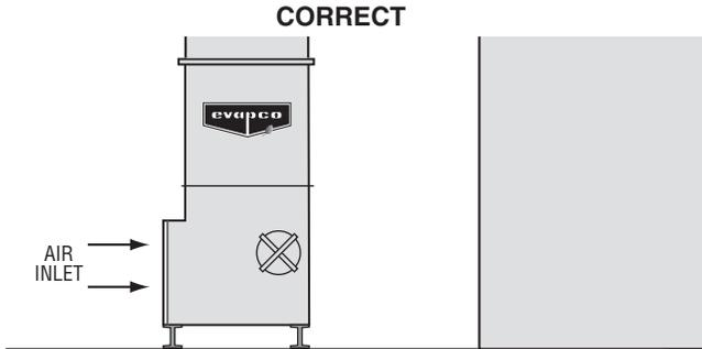
**Figure 36** - Installation with Top of Discharge Hood Above Top of Wall
