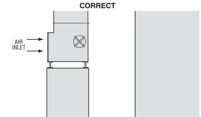
Figure 35 - Installation Elevated so Top of Unit is Higher than Top of Wall
