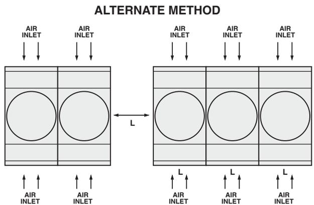
**Figure 28a - Multiple Units Placed End-to-End**
