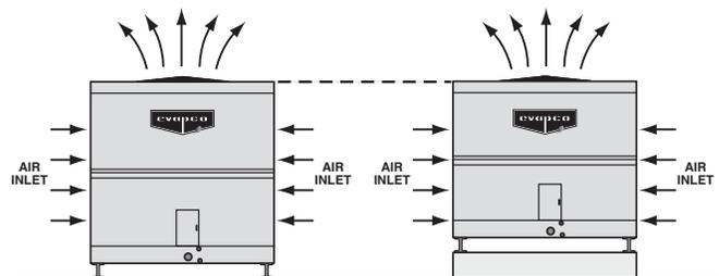
Figure 32 - Expansion to an Existing Installation
