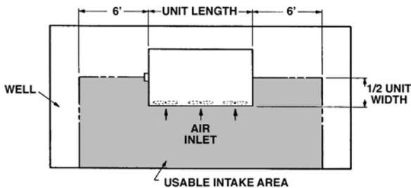
Figure 46 - Well Installation
