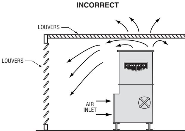
**Figure 48 - Louvered Enclosure with Grating Over Top**
