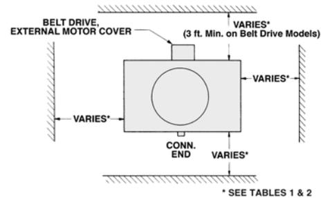
Figure 56 - Minimum Clearance Dimensions Induced Draft Counterflow Units
