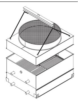
Figure 15 - Mating Fan Section to Coil Section
