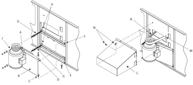
Figure 18a - External Motor Installation
