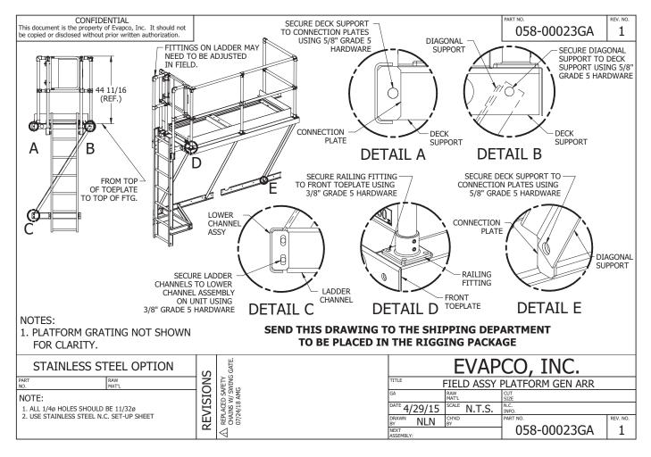
Figure 26 - Platform Mounting General Arrangement
