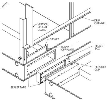
Figure 4 - Equalizer Blank-Off Plate Installation
