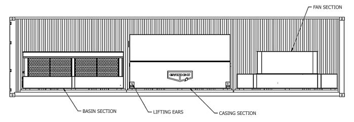
Figure 14 - 40' Standard Height Container, Unit with Super Low Sound Fan
