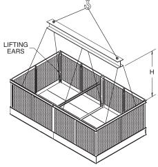
Figure 1b - Basin Section 24' (7.3m) to 40' (12.2m) long
