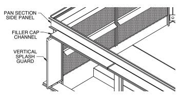
Figure 10 - Filler Cap Channel Assembly
