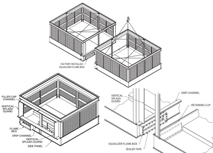
Figure 3 - Joining Bottom Sections – Multi Cell Units
