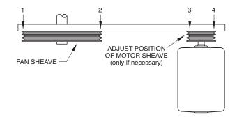
Figure 19 - Sheave Alignment Check
