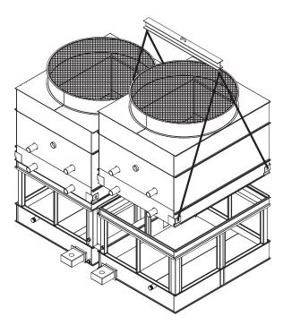
Figure 16 - Mating Fan/Coil Section to Basin Section
