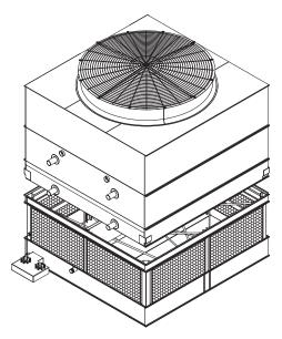
Figure 8 - Mating Upper Section to Basin Section
