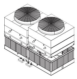
Figure 9 - Mating Upper Section to Basin Section
