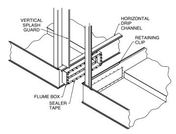
Figure 2 - Equalizer Flume Connection, 12' (3.6m) Wide Models
