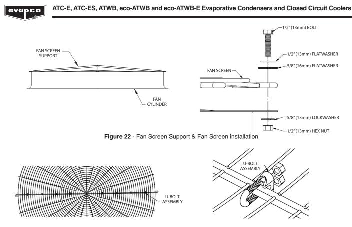
Figure 23 - U-Bolt Assembly Spacing & Arrangement
