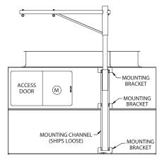
Figure 20 - Dual-Point Davit Arrangement
