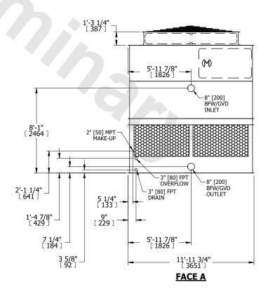
**SHIPPING** OPERATING HEAVIEST SECTION 6790 lbs+ [3080] kg+ 11750 lbs+ [5330] kg+ WEIGHT WEIGHT WEIGHT
