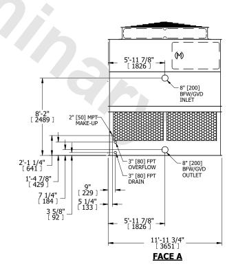
DRAWN BY: KDS NO. OF SHIPPING SECTIONS **SHIPPING** OPERATING HEAVIEST SECTION 7450 lbs+ [3380] kg+ 13660 lbs+ [6200] kg+ 5050 lbs+ [2295] kg+ WEIGHT WEIGHT WEIGHT
