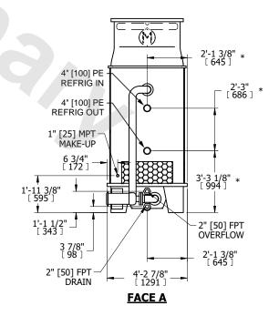
SHIPPING WEIGHT 3960 lbs+ [1800] kg+ OPERATING WEIGHT 4980 lbs+ [2260] kg+ HEAVIEST SECTION WEIGHT 3960 lbs+ [1800] kg+ NO. OF SHIPPING SECTIONS 1 DRAWN BY: JLM
