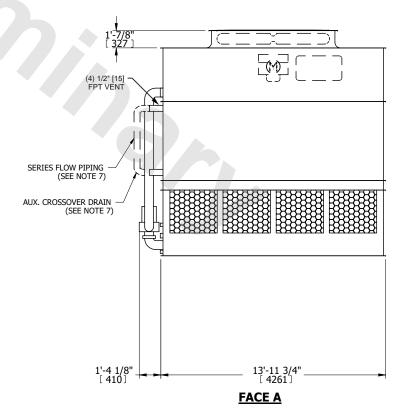
DRAWN BY: JLG NO. OF SHIPPING SECTIONS **SHIPPING OPERATING** HEAVIEST SECTION 19330 lbs+ [8770] kg+ 28270 lbs+ [12825] kg+ 17320 lbs+ [7860] kg+ WEIGHT WEIGHT WEIGHT
