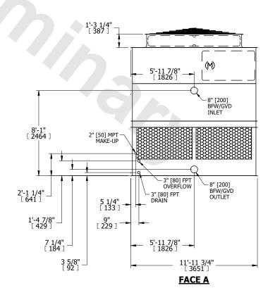
SHIPPING WEIGHT 6740 lbs+ [3060] kg+ OPERATING WEIGHT 11700 lbs+ [5310] kg+ HEAVIEST SECTION WEIGHT 4320 lbs+ [1960] kg+ NO. OF SHIPPING SECTIONS 2 DRAWN BY: JLG
