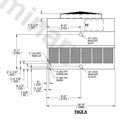
DRAWN BY: KDS NO. OF SHIPPING SECTIONS **SHIPPING** OPERATING HEAVIEST SECTION 10710 lbs+ [4860] kg+ 19980 lbs+ [9065] kg+ 6810 lbs+ [3090] kg+ WEIGHT WEIGHT WEIGHT
