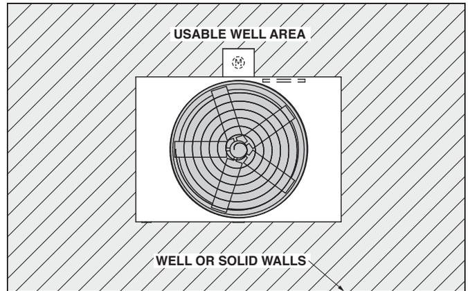
Figure 20 - Well Installation
