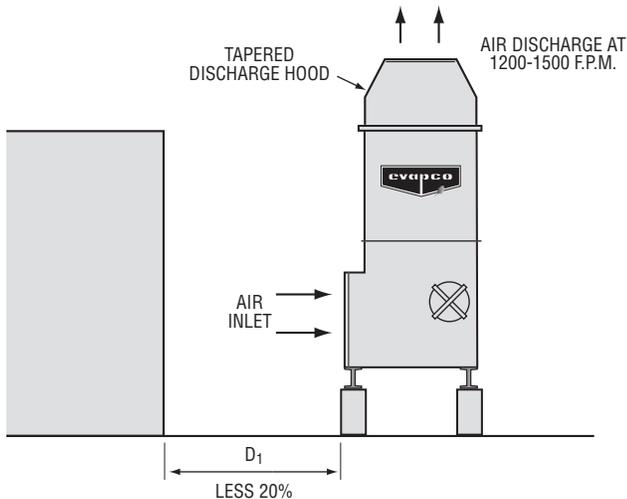
**Figure 39 - Installation with Tapered Discharge Hood**
