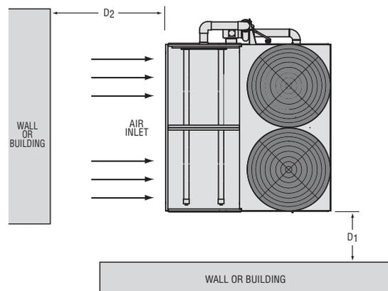
**Figure 26** - Installation Next to a Wall
