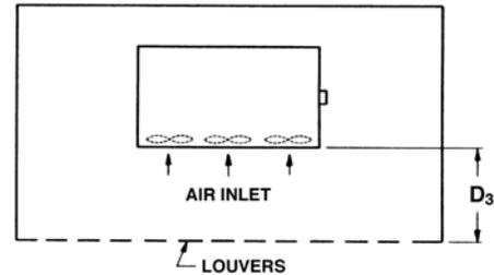
Figure 47 - Louvered Wall Enclosure with Front Louvers
