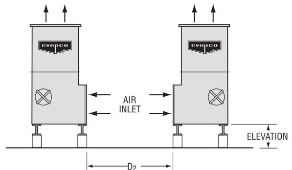
**Figure 43 - Installation with Air Inlets Facing Each Other**
