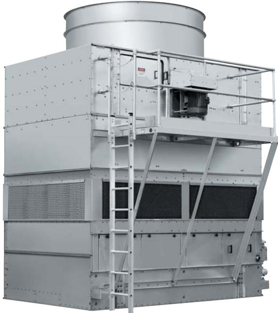
External platforms provide a sturdy base for access to the drive components, water distribution and drift eliminators. Constructed from heavy gauge galvanized steel, the platform mounts easily to the unit and requires no external support. The platform option includes a vertical aluminum ladder and meets all applicable OSHA requirements. A safety cage for the ladder is also available if required for the installation.
