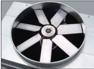
Low Sound Fan construction uses aluminum blades and a steel fan hub. The Low Sound Fan is capable of reducing the unit sound pressure levels by **4 dB(A) to 7dB(A)**, depending on specific unit selection and measurement location
