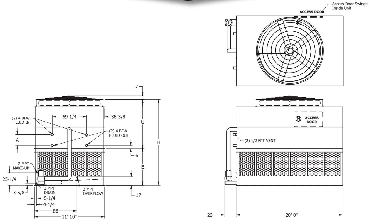
**Note:** The number of coil connections doubles when the flow rate exceeds 900 GPM on eco-ATW 12x20 models. This required option is referred to as the High Flow coil configuration.
