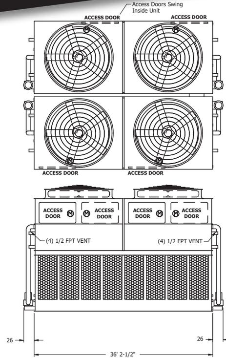
**Note:** The number of coil connections doubles when the flow rate exceeds 3,600 GPM on eco-ATW 20x36 models. This required option is referred to as the High Flow coil configuration.
