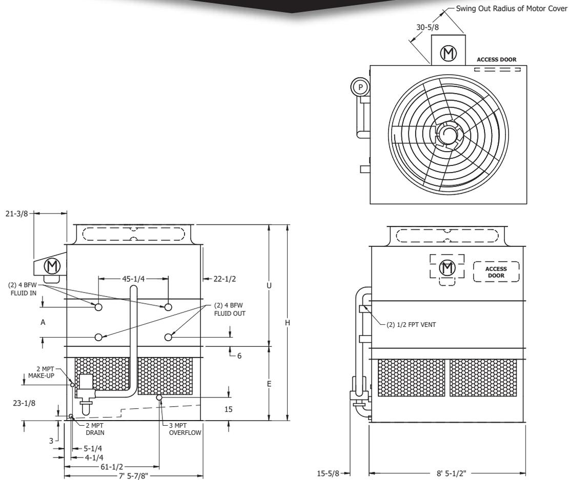
**Note:** The number of coil connections doubles when the flow rate exceeds 900 GPM on eco-ATW 9x8 models. This required option is referred to as the High Flow coil configuration.
