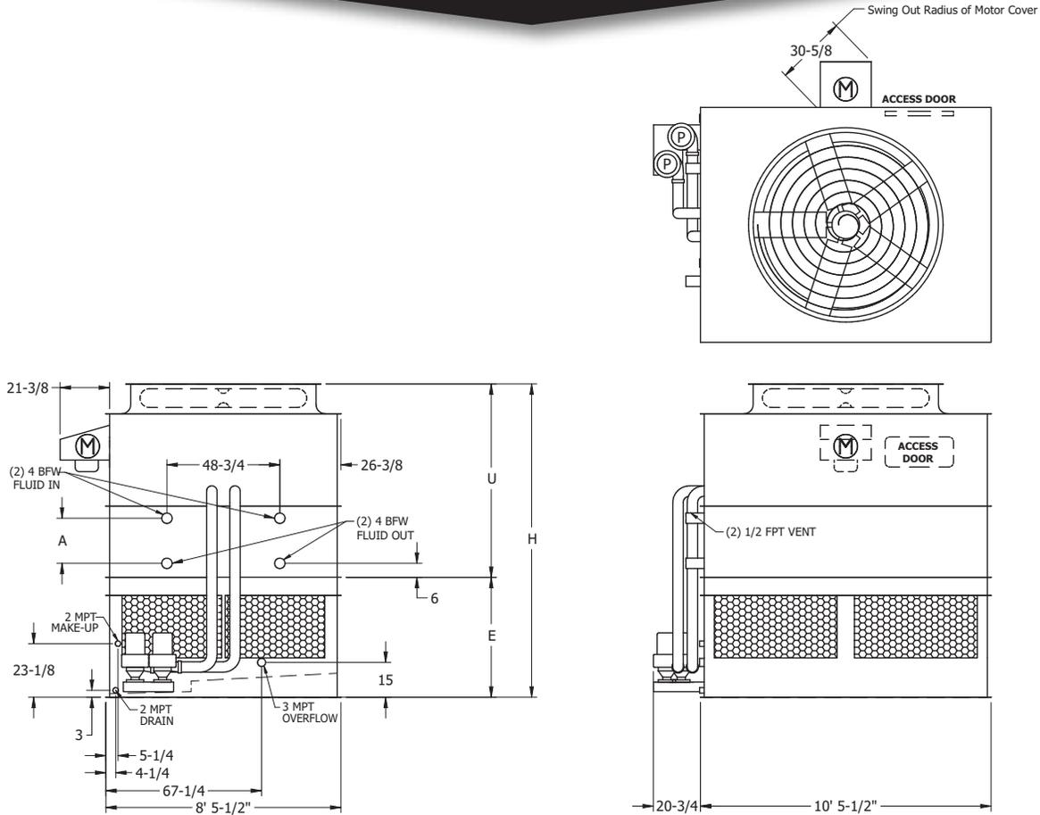
**Note:** The number of coil connections doubles when the flow rate exceeds 900 GPM on eco-ATWE 9x11 models. This required option is referred to as the High Flow coil configuration.
