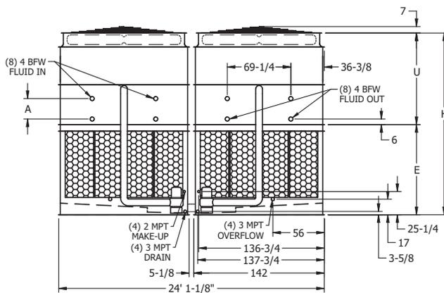
**Note:** The number of coil connections doubles when the flow rate exceeds 3,600 GPM on eco-ATC 24x40 models. This required option is referred to as the High Flow coil configuration.
