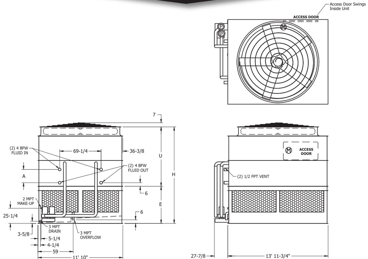
**Note:** The number of coil connections doubles when the flow rate exceeds 900 GPM on eco-ATWE 12x14 models. This required option is referred to as the High Flow coil configuration.
