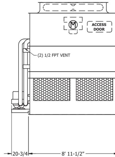
**Note:** The number of coil connections doubles when the flow rate exceeds 900 GPM on eco-ATWE 9x9 models. This required option is referred to as the High Flow coil configuration.
