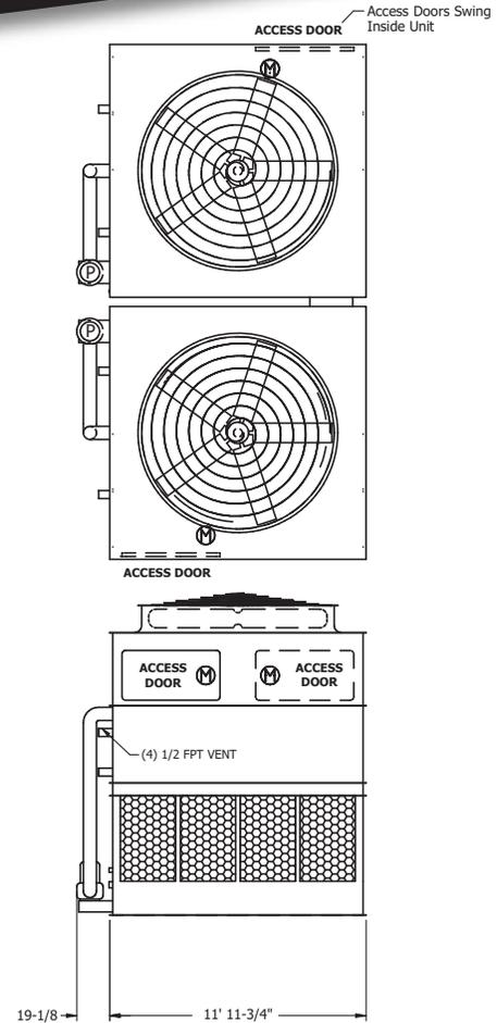
**Note:** The number of coil connections doubles when the flow rate exceeds 1,800 GPM on eco-ATW 24x12 models. This required option is referred to as the High Flow coil configuration.
