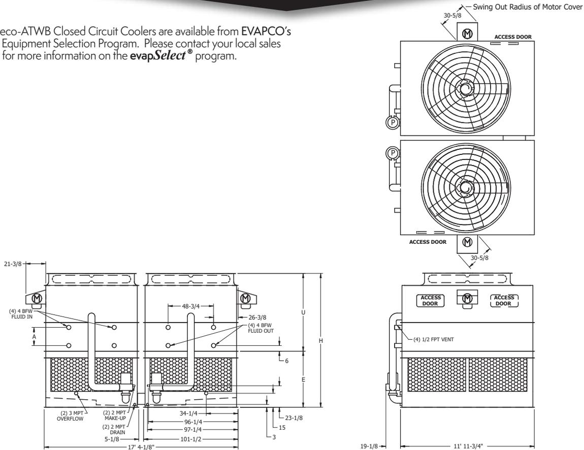
**Note:** The number of coil connections doubles when the flow rate exceeds 1,800 GPM on eco-ATW 17x12 models. This required option is referred to as the High Flow coil configuration.
