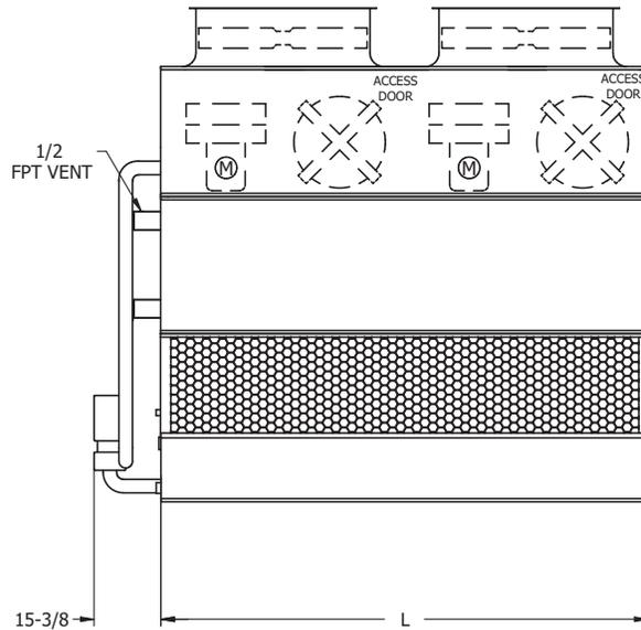
**Note:** The number of coil connections doubles when the flow rate exceeds 450 GPM on eco-ATW 4x9 and 4x12 models. This required option is referred to as the High Flow coil configuration.
