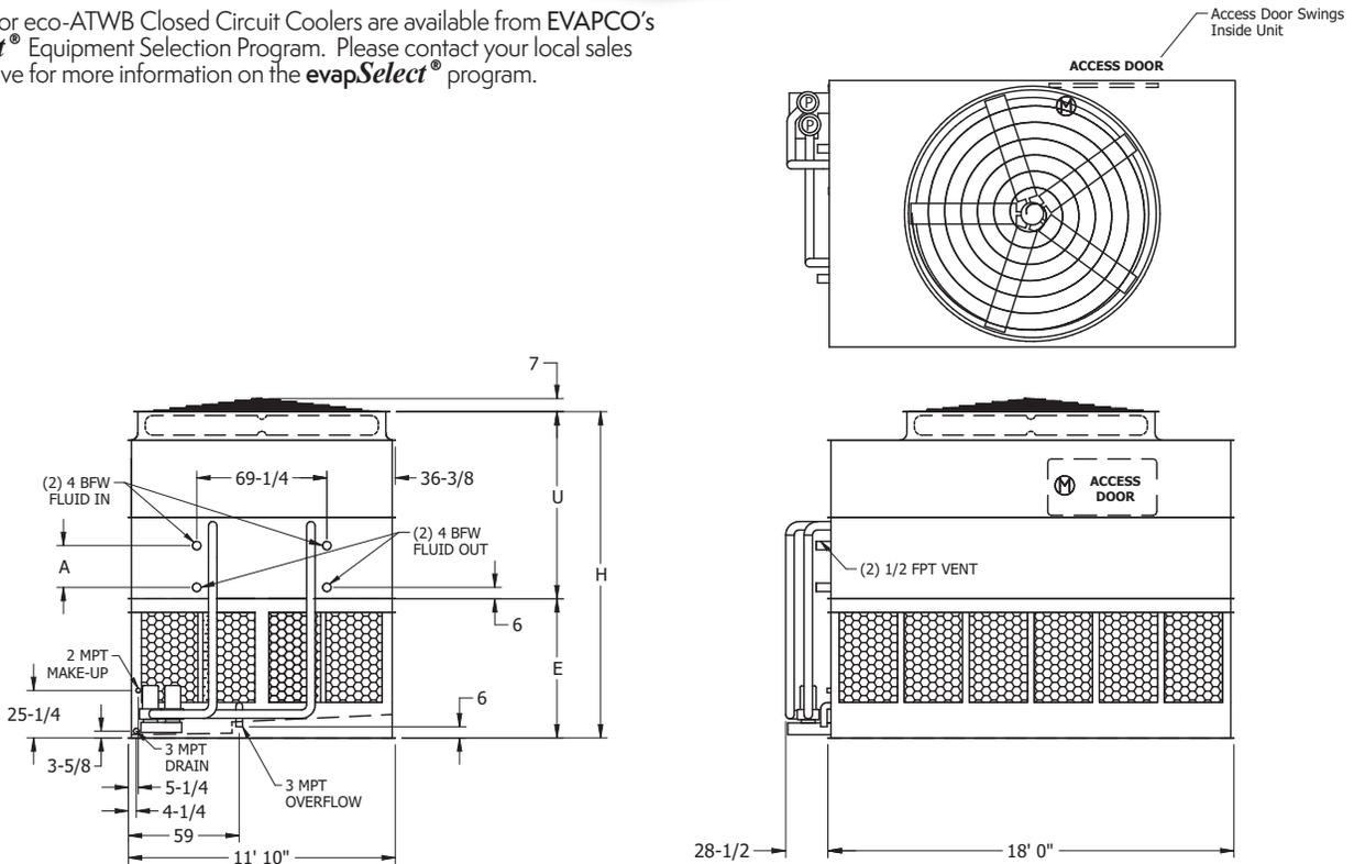
**Note:** The number of coil connections doubles when the flow rate exceeds 900 GPM on eco-ATWE 12x18 models. This required option is referred to as the High Flow coil configuration.
