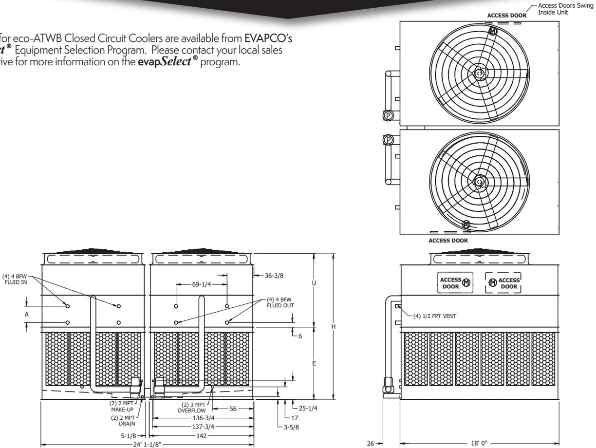
**Note:** The number of coil connections doubles when the flow rate exceeds 1,800 GPM on eco-ATW 24x18 models. This required option is referred to as the High Flow coil configuration.
