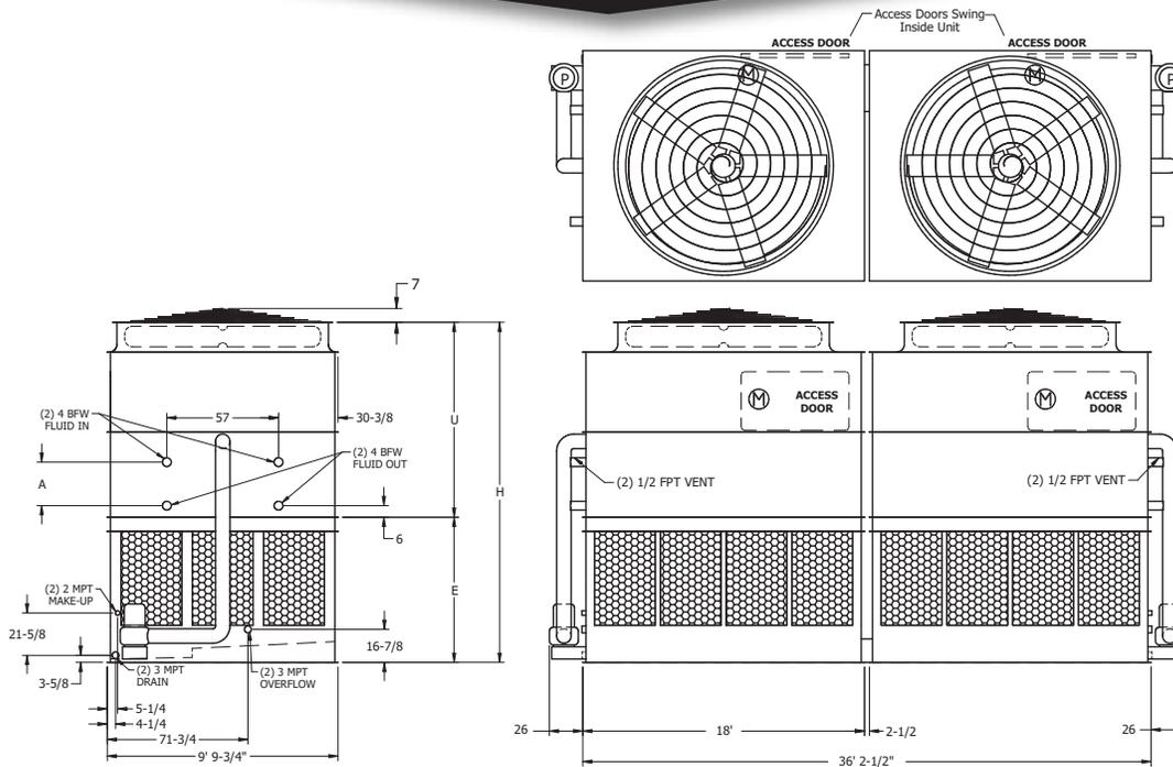
**Note:** The number of coil connections doubles when the flow rate exceeds 1,800 GPM on eco-ATW 10x36 models. This required option is referred to as the High Flow coil configuration.
