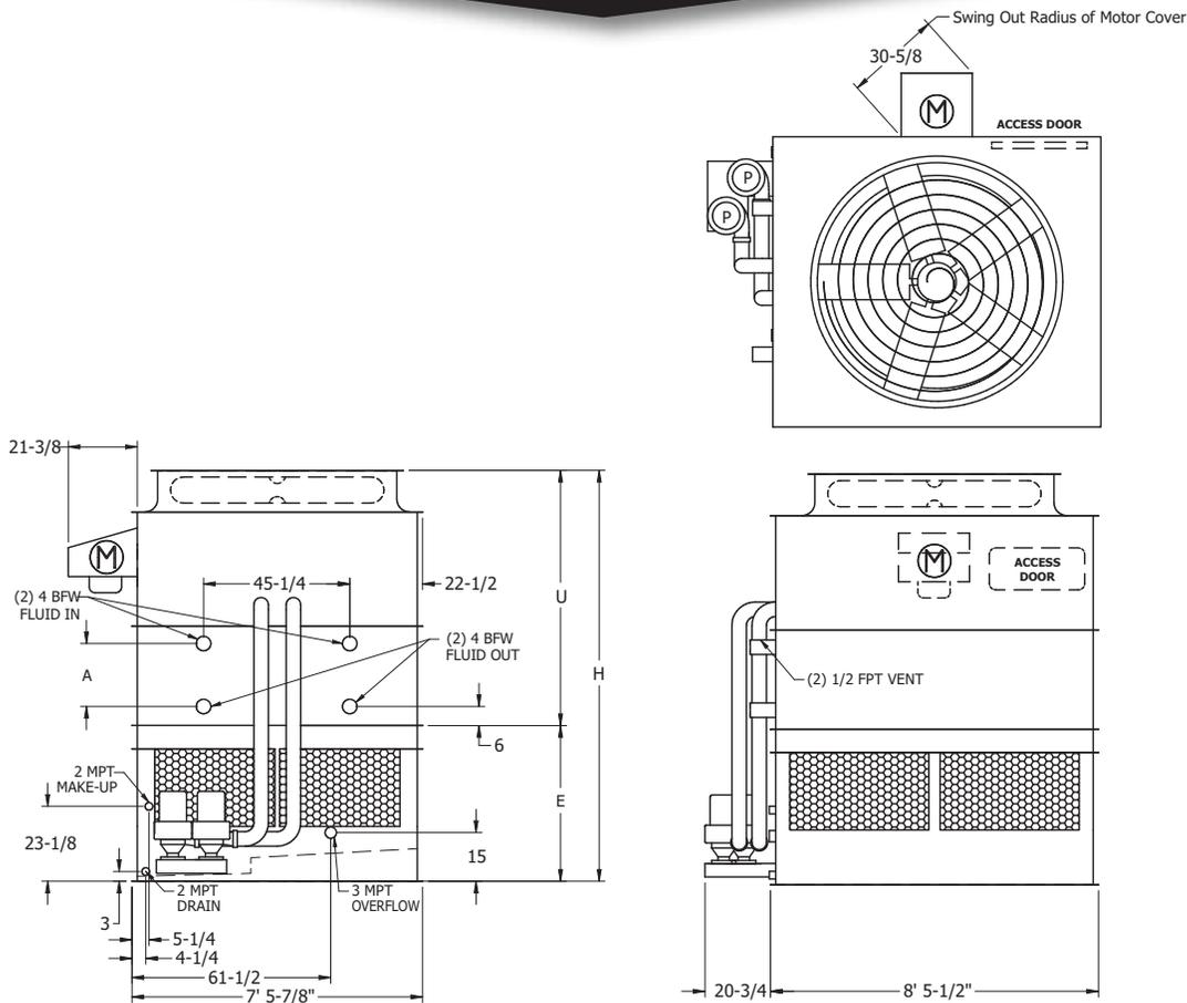
**Note:** The number of coil connections doubles when the flow rate exceeds 900 GPM on eco-ATWE 9x8 models. This required option is referred to as the High Flow coil configuration.
