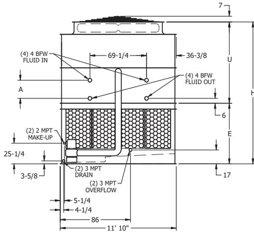
**Note:** The number of coil connections doubles when the flow rate exceeds 1,800 GPM on eco-ATW 12x24 models. This required option is referred to as the High Flow coil configuration.
