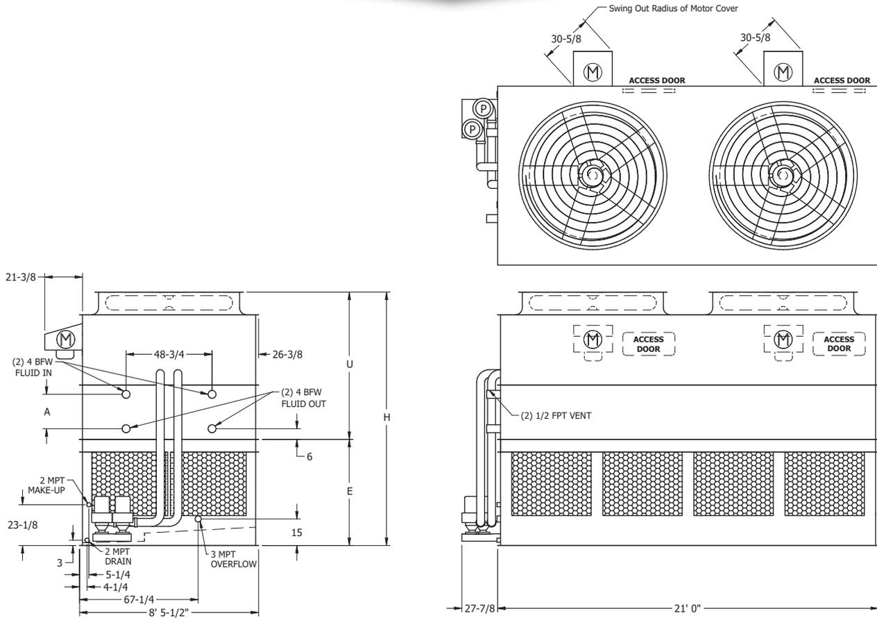
**Note:** The number of coil connections doubles when the flow rate exceeds 900 GPM on eco-ATWE 9x21 models. This required option is referred to as the High Flow coil configuration.
