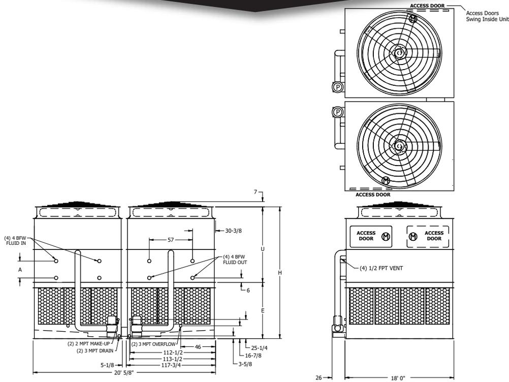
**Note:** The number of coil connections doubles when the flow rate exceeds 1,800 GPM on eco-ATW 20x18 models. This required option is referred to as the High Flow coil configuration.
