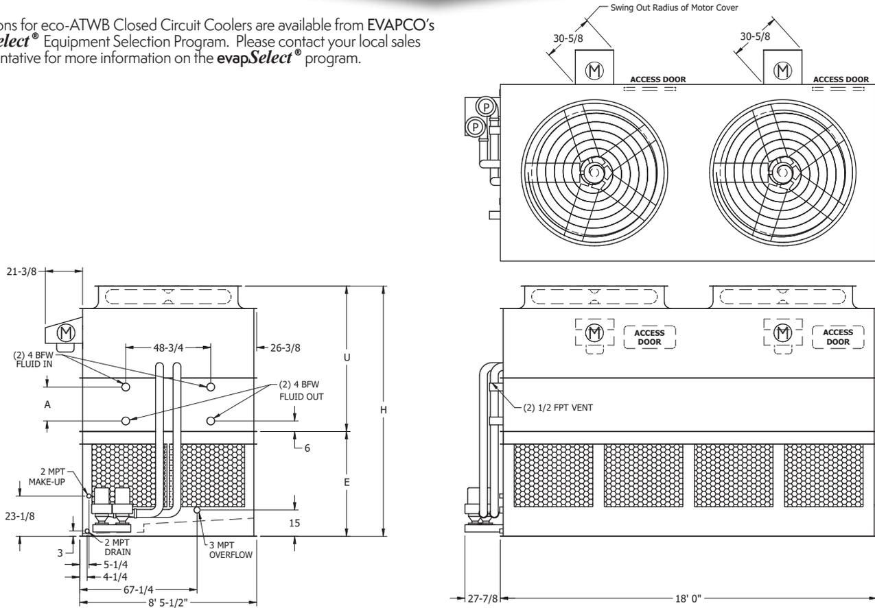
**Note:** The number of coil connections doubles when the flow rate exceeds 900 GPM on eco-ATWE 9x18 models. This required option is referred to as the High Flow coil configuration.
