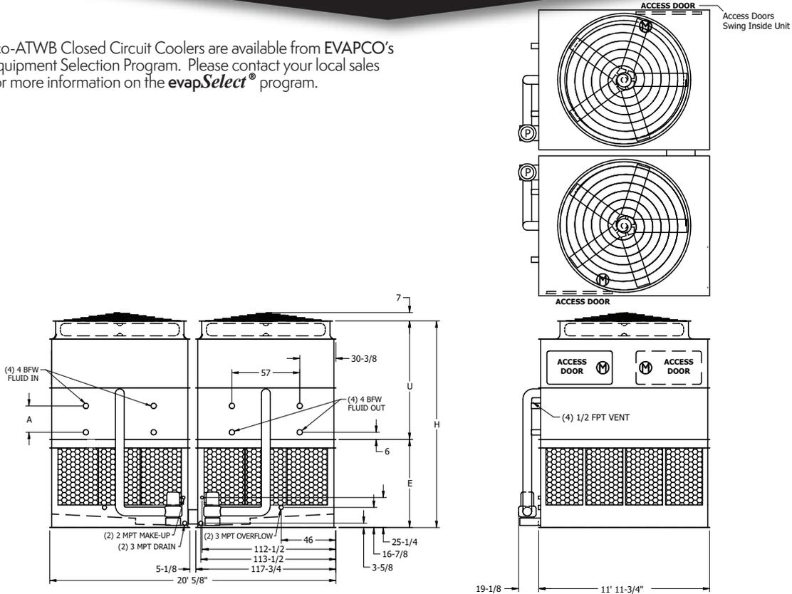
**Note:** The number of coil connections doubles when the flow rate exceeds 1,800 GPM on eco-ATW 20x12 models. This required option is referred to as the High Flow coil configuration.
