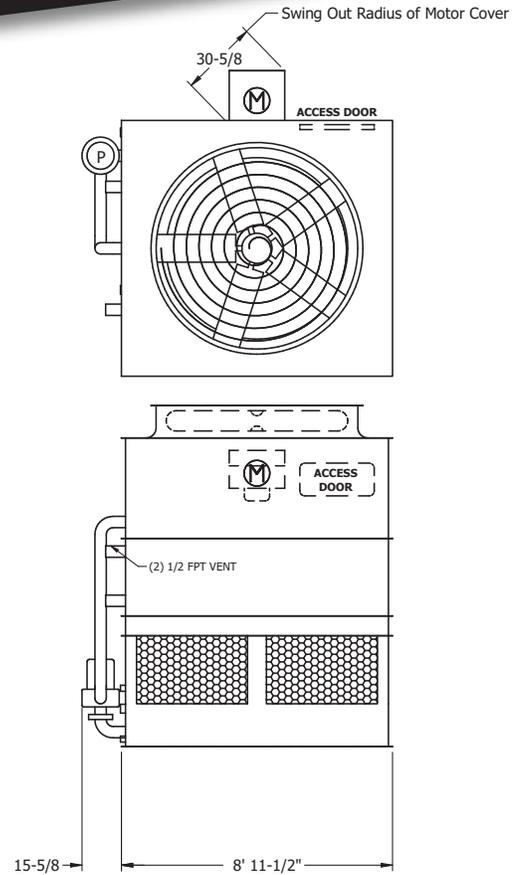
**Note:** The number of coil connections doubles when the flow rate exceeds 900 GPM on eco-ATW 9x9 models. This required option is referred to as the High Flow coil configuration.
