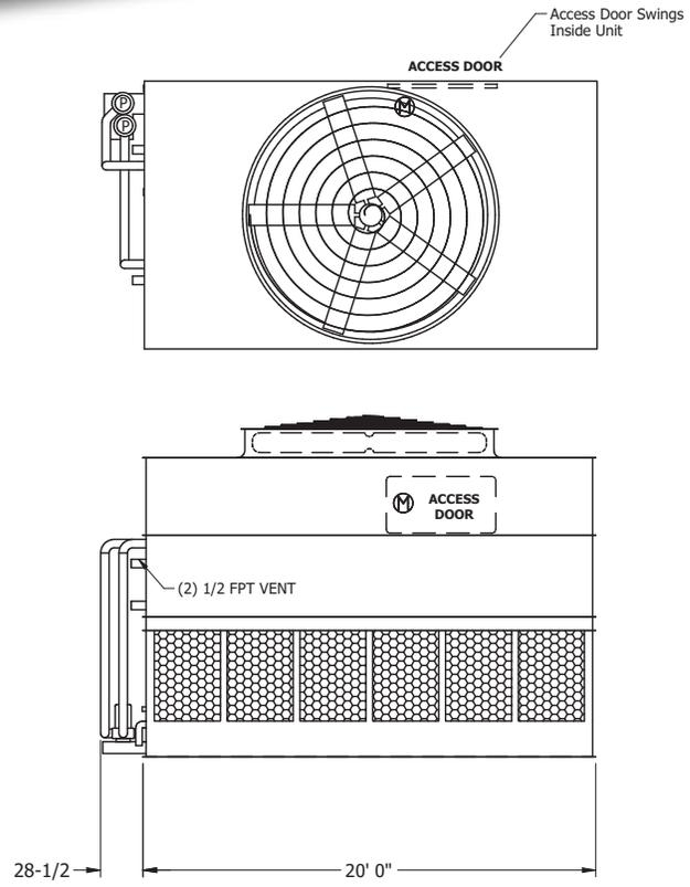
**Note:** The number of coil connections doubles when the flow rate exceeds 900 GPM on eco-ATWE 12x20 models. This required option is referred to as the High Flow coil configuration.
