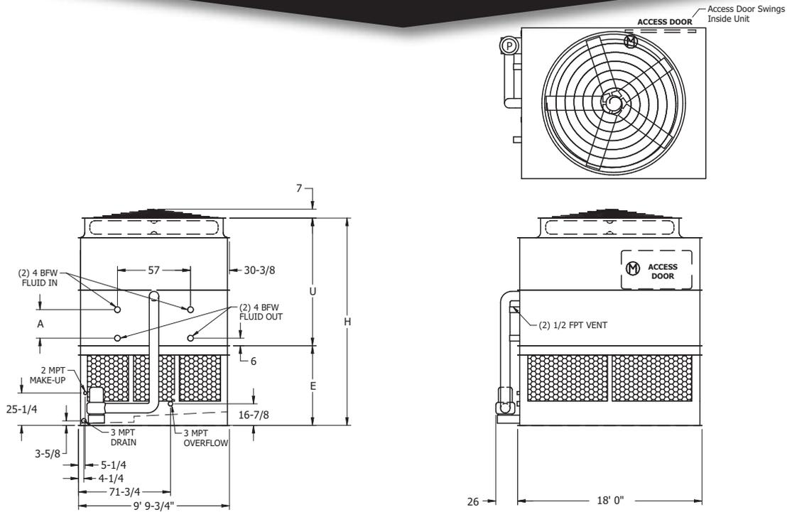
**Note:** The number of coil connections doubles when the flow rate exceeds 900 GPM on eco-ATW 10x18 models. This required option is referred to as the High Flow coil configuration.
