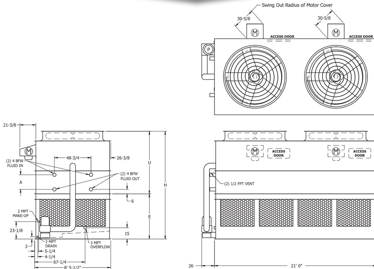
**Note:** The number of coil connections doubles when the flow rate exceeds 900 GPM on eco-ATW 9x21 models. This required option is referred to as the High Flow coil configuration.
