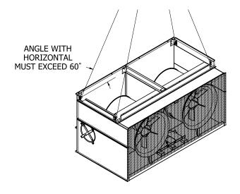
Figure 2 - Pan - Fan Section (up to 20' Long)
