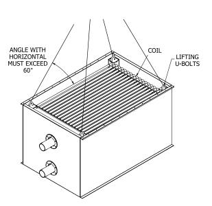
Figure 7 - Small, Single Coil Sections (PMC-175E to 375E)
