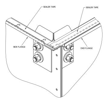
Figure 5 - Proper Sealer Tape Application
