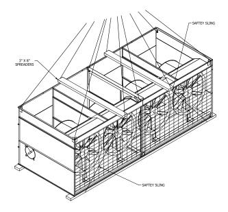
Figure 4 - Proper Rigging Method for Extended Lifts
