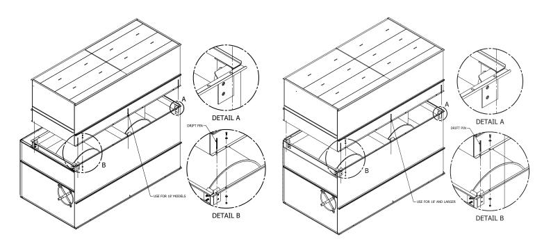
Figure 10 - Mating Upper Section to Basin Section (PMC-250E to 375E)
