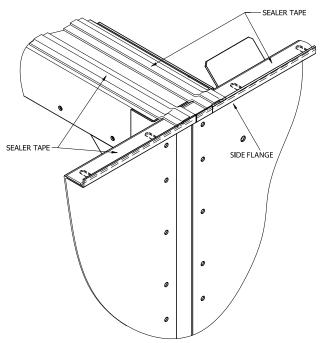
Figure 6 - Sealer Detail for Center Joint of Units with two Coil Sections
