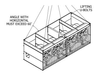
Figure 3 - Pan - Fan Section (over 20' Long)
