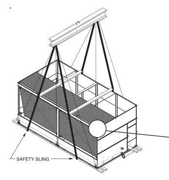
Figure 6 - Proper Rigging Method for Extended Lifts
