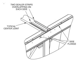
Figure 8 – Sealer Detail for Center End Flange Joint of S and L Models with 18' or 24' Coil Sections
