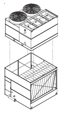
Figure 12 - Mating Upper Coil / Fan Section to Basin Section
