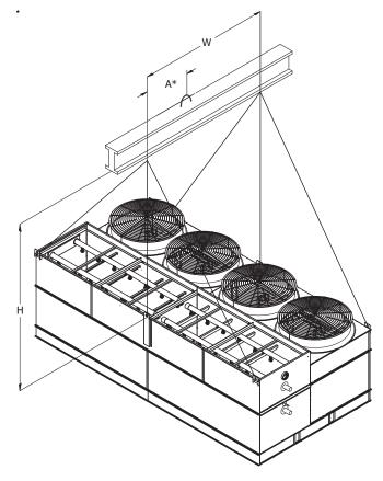
Figure 10 – L Model Coil / Fan Section – 24' Long
