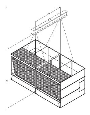
Figure 4 - L Model Basin Section - 24' Long
