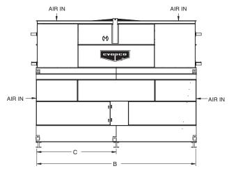
Figure 1 - Recommended Steel Support for S and L Models
