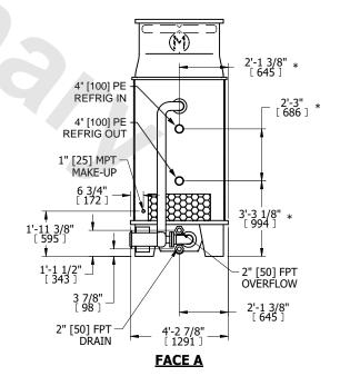
SHIPPING WEIGHT 3910 lbs+ [1775] kg+ OPERATING WEIGHT 4930 lbs+ [2240] kg+ HEAVIEST SECTION WEIGHT 3910 lbs+ [1775] kg+ NO. OF SHIPPING SECTIONS 1 DRAWN BY: JLM
